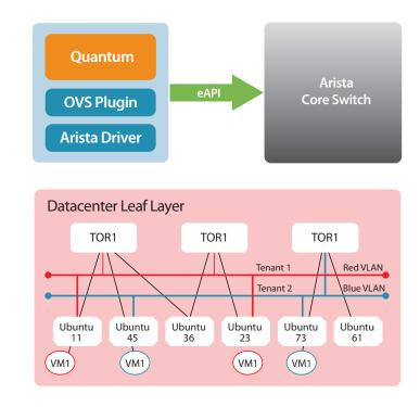
The figure above shows two OpenStack tenant networks (Red Network and Blue Network) for which corresponding Quantum networks have been provisioned. The OVS plugin decides on the VLAN allocation for these tenant networks - Red VLAN and Blue VLAN above. These VLAN choices are conveyed by the OVS plugin to the Arista driver.
