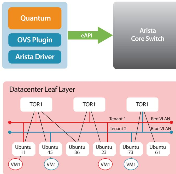
The figure above shows two OpenStack tenant networks (Red Network and Blue Network) for which corresponding Quantum networks have been provisioned. The OVS plugin decides on the VLAN allocation for these tenant networks - Red VLAN and Blue VLAN above. These VLAN choices are conveyed by the OVS plugin to the Arista driver.
